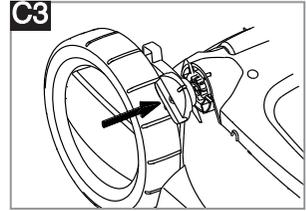
3. Insert the Pivot Block on to the Bolt (**C3**)
